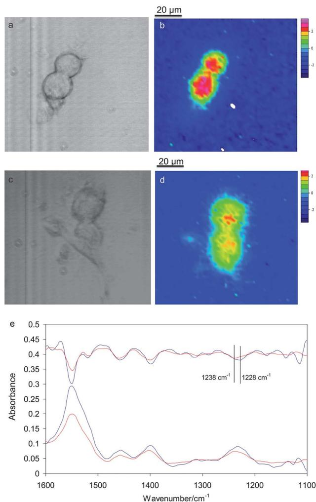
**Fig. 4** Visible (a and c) and FTIR (b and d) images (generated using the amide II band at  $1545\text{ cm}^{-1}$ ) of a few adjacent cells. Images (a) and (b) are captured immediately after injecting the cells into the device, images (c) and (d) are captured after cells have started to spread. (e) Averaged spectra from cells (bottom) and their corresponding 2<sup>nd</sup> derivatives spectra (top) before (blue lines) and after (red lines) spreading.
